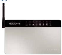
EzLogger Pro is a self-developed monitoring device by GoodWe. In combination with a GoodWe solar inverter, it can easily read and record all key plant data and constantly transmit the data to the GoodWe portal via internet.
